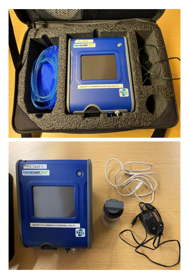
**Construct as follows:** Connect power cable in back of Portacount and plug into mains power.
