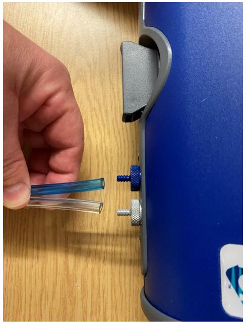
c) Remove storage cap from front of the Portacount and remove alcohol wick and insert into the front of Portacount ensuring excess alcohol is not on the wick. Put cap on Alcohol cartridge as lid.
