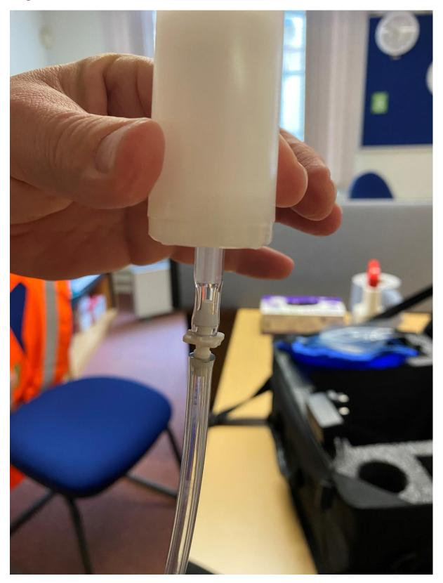
Max Fit test: Completed by fit plus software to make sure Portacount can measure high fit factors and internal switch valve is functioning properly.
