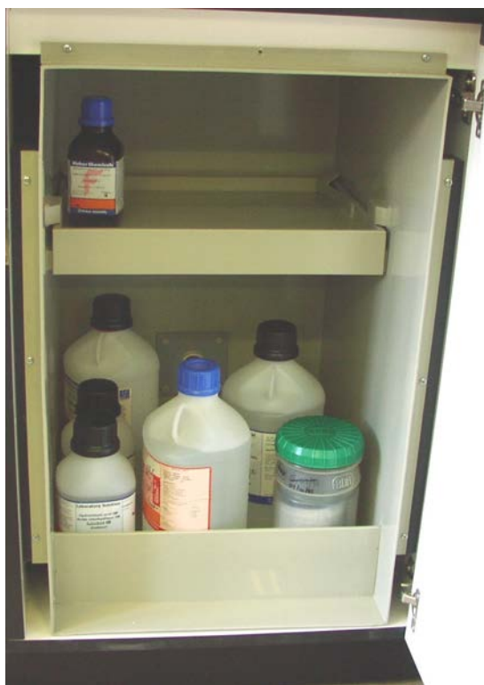
Figure 4 – Bottles stored in drip trays within ventilated acids cabinet including example of chemically resistant secondary containment (BDH / VWR Safepak bottom right)
