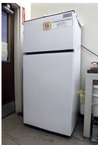
Figure 1 – Modified domestic-type refrigerator used to store chemicals
